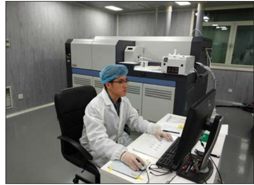
Oliver running samples on the MC-ICPMS to measure U-Th isotopes
