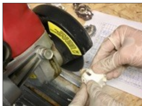
Alicia cutting the shell of Crassostrea gigas to reveal growth rings
