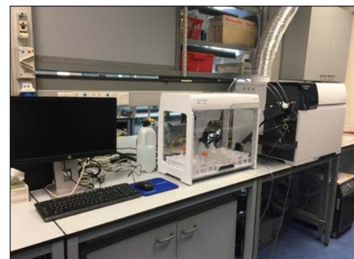
ICP-MS used for trace element measurement in ostracods
