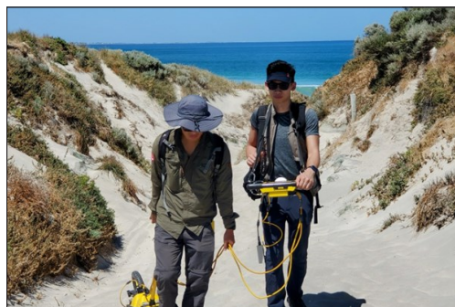
Howard running ground penetrating radar transects with collaborators from NTU in Western Australia
