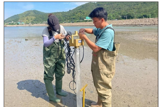
Mandy and Bovern setting up a sediment corer to collect sediment samples from seagrass bed sediment
