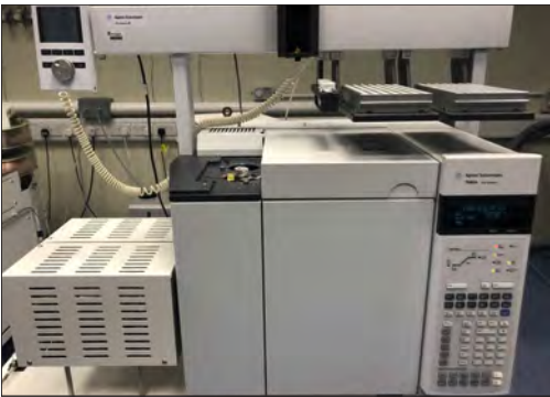
The GC-C-IRMS used by Taihun in the SIRMS Laboratory
