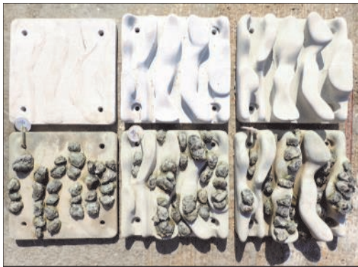
Habitat tiles being used to test if provision of microhabitats can enhance biodiversity on seawalls
