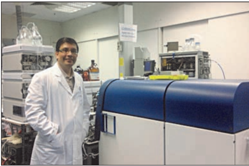
Joy with the LC-MS/MS Mass spectrometer instrument (AB Sciex Triple TOF 5600 system) dedicated for the proteomics laboratory
